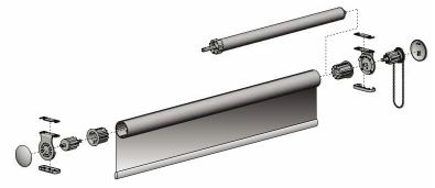
The SP60/80 Heavy Duty roller blind system can be controlled by chain, motor or crank. Its chain control is designed to lift blinds of up to 25 kg while maintaining a strong pull force of less than 3 kg. The motors can be controlled by wall remote, hand-held remote, Smartphone App, Home Automation System (HAS) or Building Management System (BMS).
