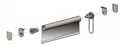
The SP45 roller blind system is designed for commercial and residential use. It is the smart and modern solution to light and privacy control. SP45 roller blinds can be motorised and controlled by remote, Smartphone App, Home Automation System (HAS) or Building Management System (BMS). Up to 3 blinds can be linked together to one chain or one motor. Its chain control is designed to lift blinds of up to 9 kg while maintaining a strong pull force of less than 3 kg.
